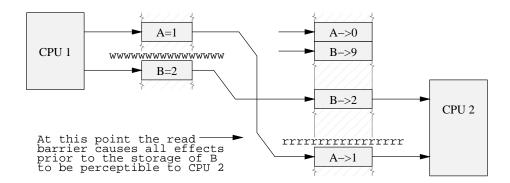
Figure 11.11: Read Barrier Supplied
