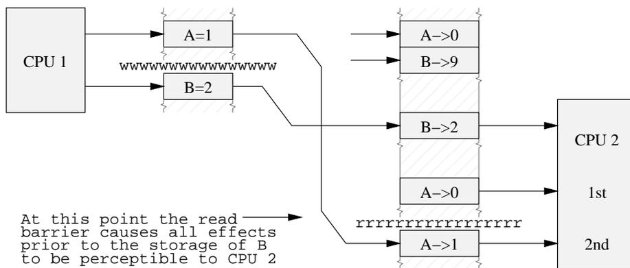
Figure 11.12: Read Barrier Supplied, Double Load
