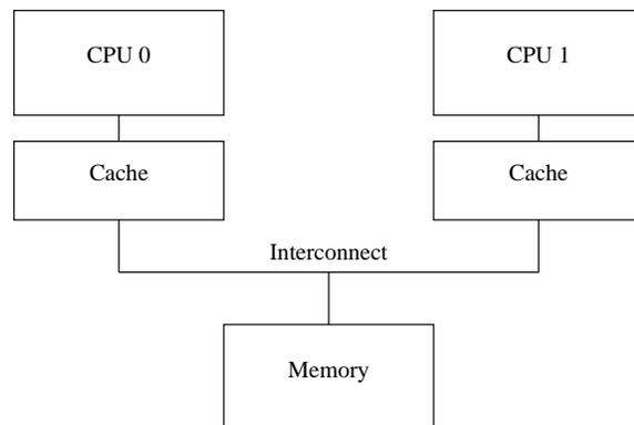
Figure 11.1: Modern Computer System Cache Structure
