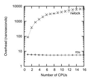
Figure 8.16: Performance Advantage of Preemptable RCU Over Reader-Writer Locking
