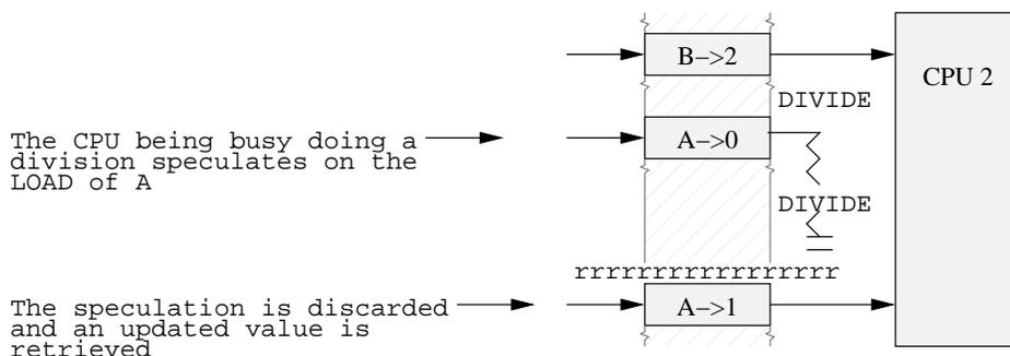
Figure 11.16: Speculative Load Cancelled by Barrier
