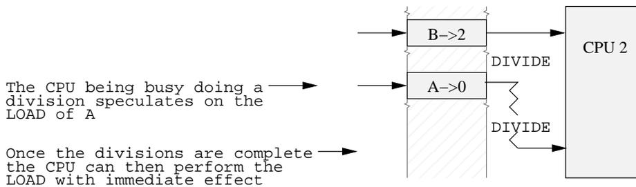
Figure 11.14: Speculative Load
