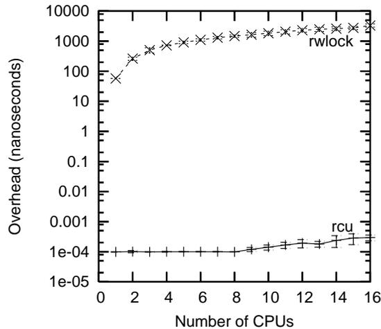
Figure 8.15: Performance Advantage of RCU Over Reader-Writer Locking
