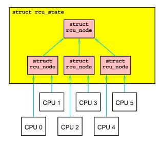
Figure D.12: Hierarchical RCU State
