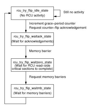
Figure D.63: Preemptable RCU State Machine
