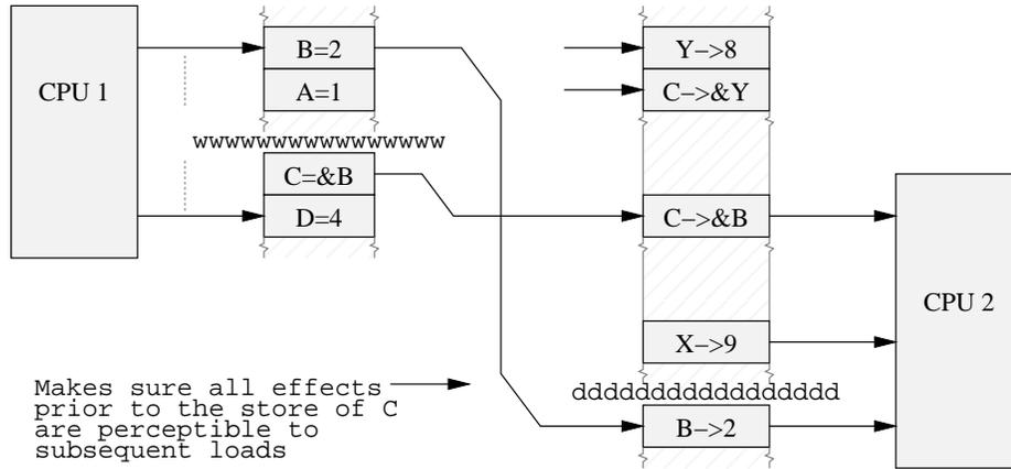
Figure 11.9: Data Dependency Barrier Supplied
