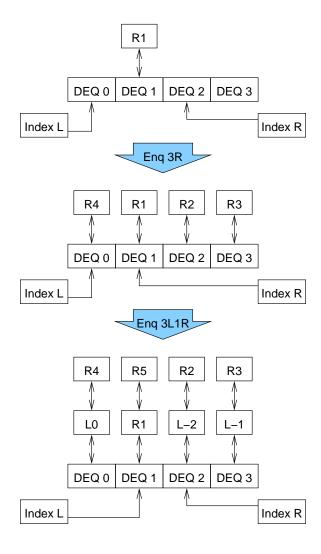
Figure 5.7: Hashed Double-Ended Queue After Insertions
