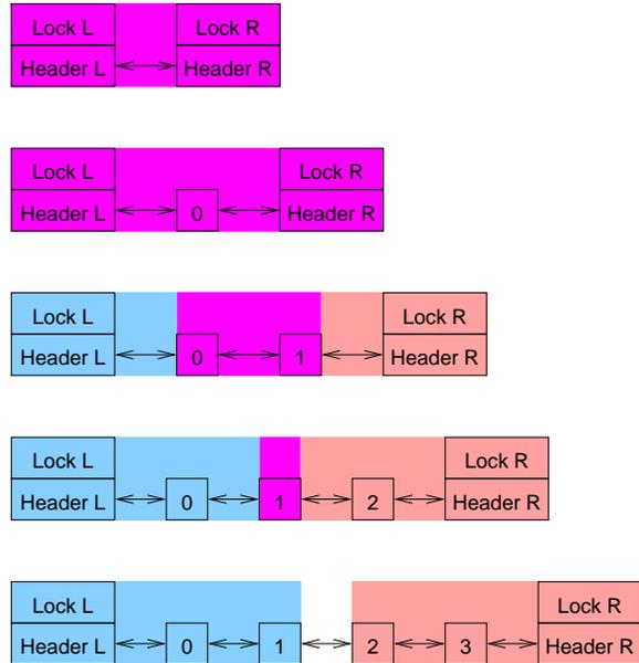
Figure 5.4: Double-Ended Queue With Left- and Right-Hand Locks
