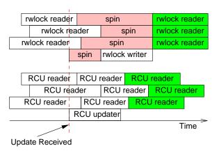
Figure 8.18: Response Time of RCU vs. Reader-Writer Locking
