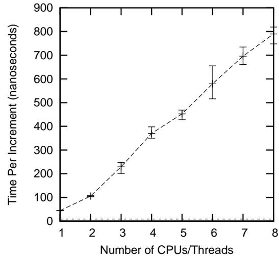
Figure 4.3: Atomic Increment Scalability on Nehalem
