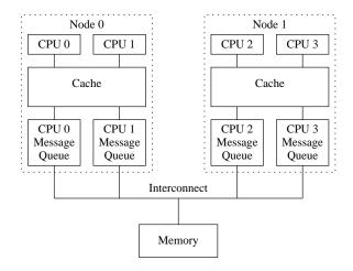
Figure C.8: Example Ordering-Hostile Architecture
