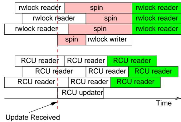
Figure 8.18: Response Time of RCU vs. Reader-Writer Locking
