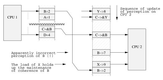
Figure 11.8: Data Dependency Barrier Omitted
