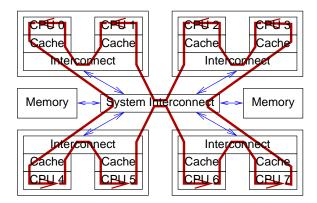
Figure 4.4: Data Flow For Global Atomic Increment
