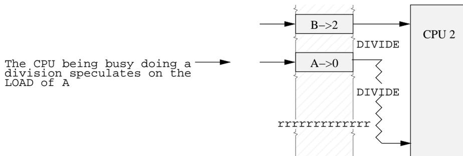
Figure 11.15: Speculative Load and Barrier
