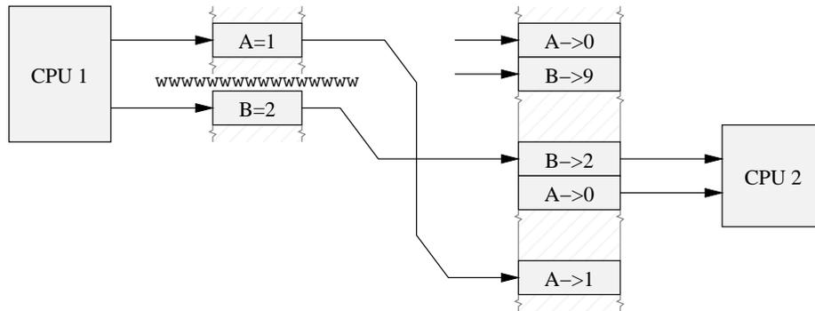
Figure 11.10: Read Barrier Needed
