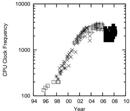
Figure 5.13: Clock-Frequency Trend for Intel CPUs
