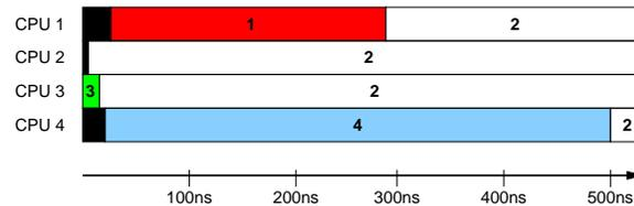
Figure 11.5: A Variable With Multiple Simultaneous Values
