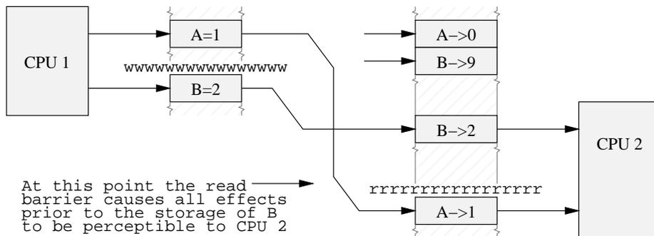
Figure 11.11: Read Barrier Supplied
