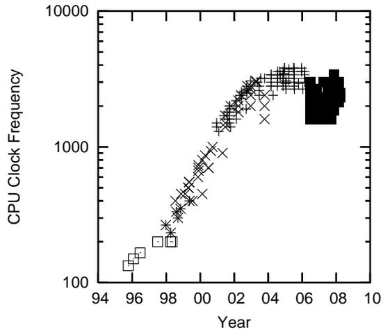
Figure 1.1: Clock-Frequency Trend for Intel CPUs
