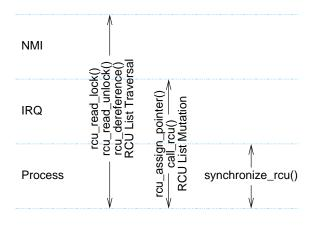
Figure 8.28: RCU API Usage Constraints
