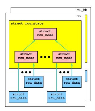
Figure D.16: Hierarchical RCU State With BH
