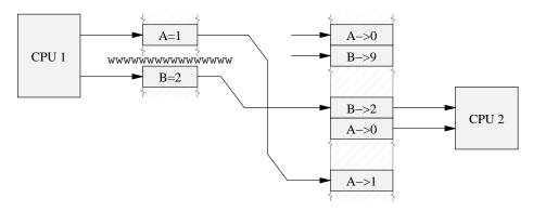
Figure 11.10: Read Barrier Needed
