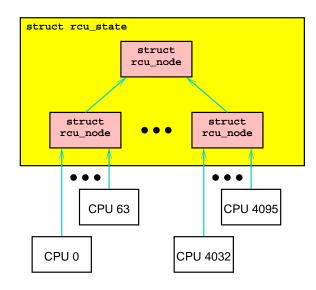
Figure D.15: Hierarchical RCU State 4,096 CPUs
