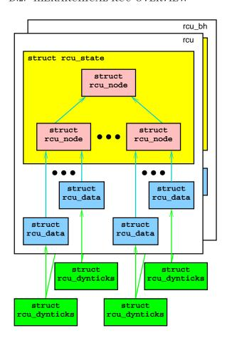
Figure D.17: Hierarchical RCU State With Dynticks
