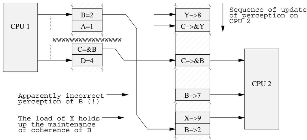
Figure 11.8: Data Dependency Barrier Omitted
