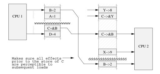
Figure 11.9: Data Dependency Barrier Supplied
