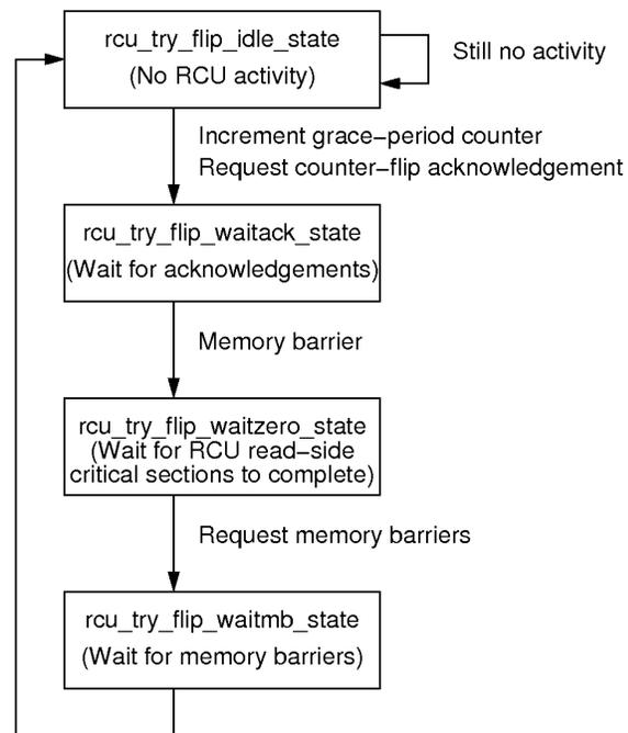
Figure D.63: Preemptable RCU State Machine
